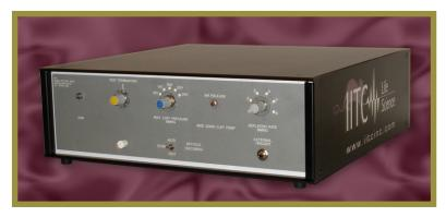
in 10-15 seconds. Single or repetitive cycles with extremely linear deflation rates. A manual air release is for immediate pressure drop. A built-in recycle timer can be set to automatically inflate the system in increments of 1 to 999 seconds.
