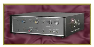
Analog output. The instrument has separate outputs for single channel and dual channel (superimposed and split) recording. The typical pulse amplitude is 100 mV to 1 V. The pressure amplitude is adjustable from one to five volts at 300 mmHg. If systolic and heart rate are desired, a single channel chart recorder #38L is sufficient. If the Mean and Diastolic are the desired reading then a dual channel chart recorder is recommended #45L or the IITC software package #31.
