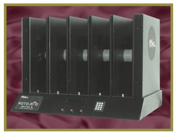
The LED display shows all test results for each animal position; they are: Stopping RPM, length of test and distance traveled.
